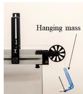
Figure 4: Hanging Mass Before Release
