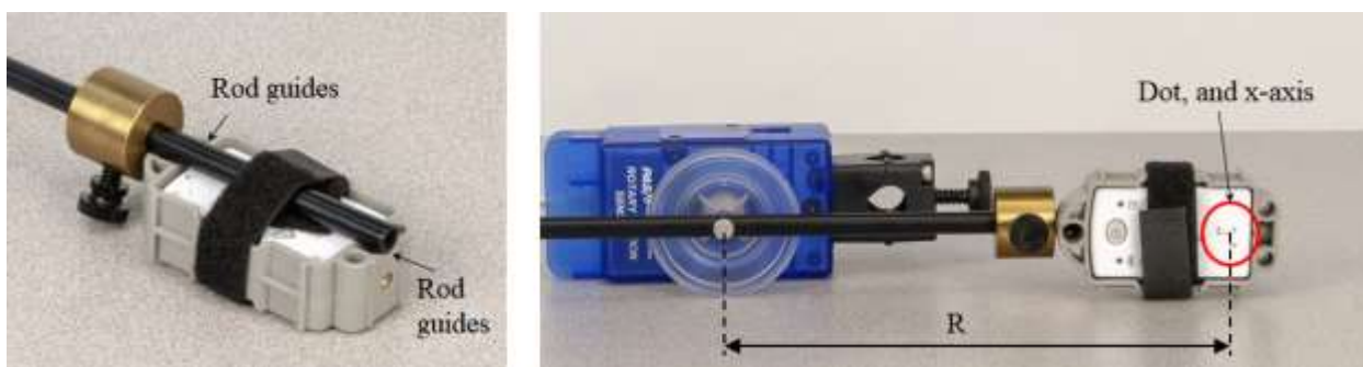
Figure 3: Attaching WAS to Pendulum Rod
