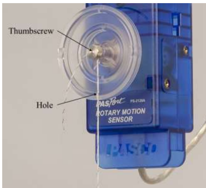
Figure 2: Attaching the string to the Rotary Motion Sensor
