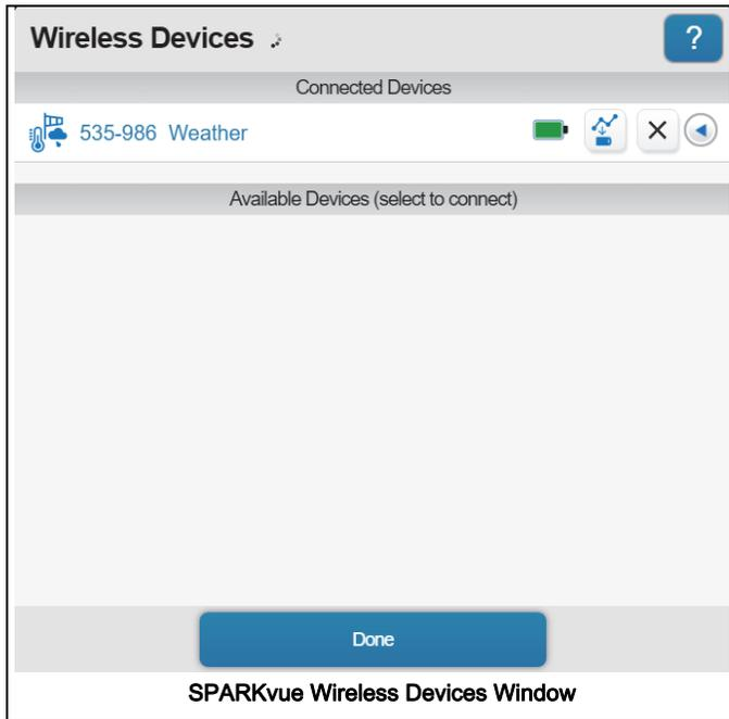
Select the “Available Device” that has the same six-digit Device ID as the one on the sensor. Select “Done”.
