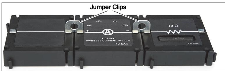
**Usage:** Use Jumper Clips to connect the Current Sensor Module as part of a circuit of other modules to measure the current through the circuit.
