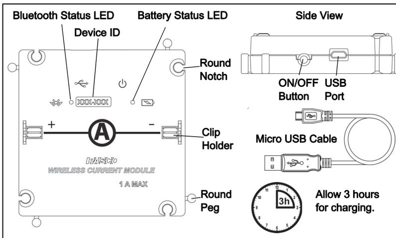
**INITIAL STEP - Connect and charge it:** Use the micro USB cable to connect the module to a USB port or a USB charger (such as PS-3501). If the cable is connected to a USB port or a USB charger, the Battery status LED shines yellow to show that the battery is charging. When the battery is charged, the Battery status LED shines green. Expect charging to take 3 hours.
