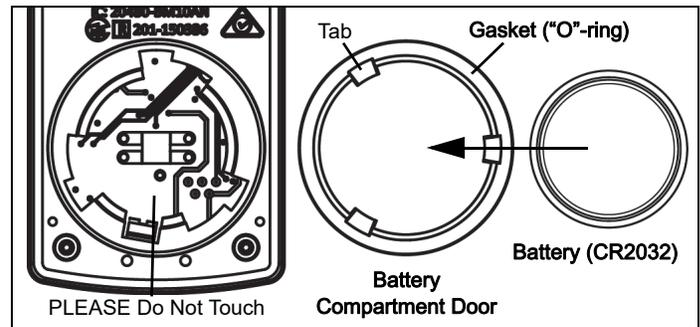
Remove the used battery from the Battery Compartment Door and replace it with a new identical type battery.
