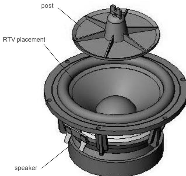
**Figure 1. Alignment of Post on Speaker**
