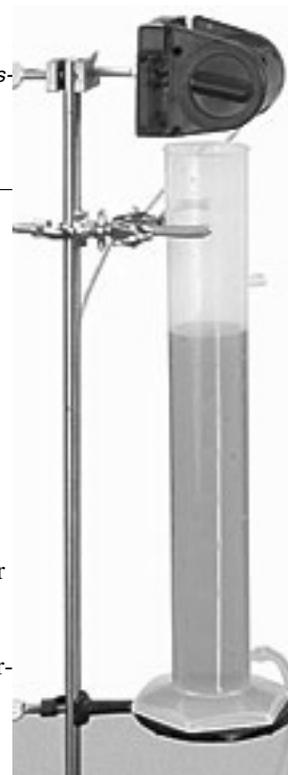
Figure 9: Motion sensor and water reservoir
