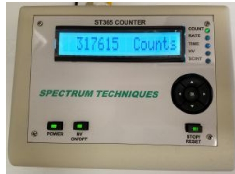
ST365B 16 Digit LCD on right.
