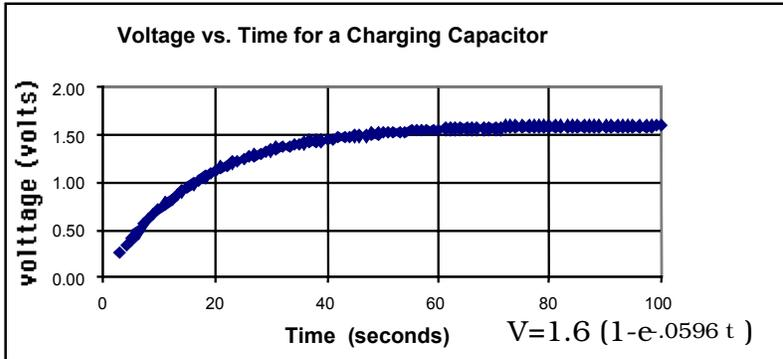
11. The actual capacitance was .00110 Farads compared to .00100 Farads printed on the capacitor.
