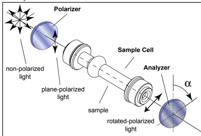
The data collection software produces a graph of light intensity compared to angle, and can be used to analyze the data to determine various properties of the optically active substance.
