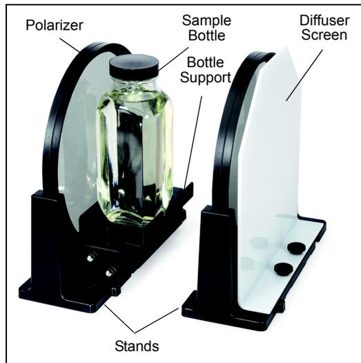
Fill a sample bottle with an optically active substance such as corn syrup and place it on the bottle support between the two polarizers. Shine a light through the diffuser screen, polarizer, and the sample bottle. Adjust the second polarizer to measure the angle of rotation.
