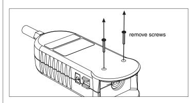
2. Firmly pull apart the halves of the enclosure. As you open the AirLink, the circuit board will separate from the top half of the enclosure.
