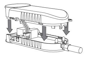
**14.** Align the halves of the AirLink and press firmly to snap them together.
