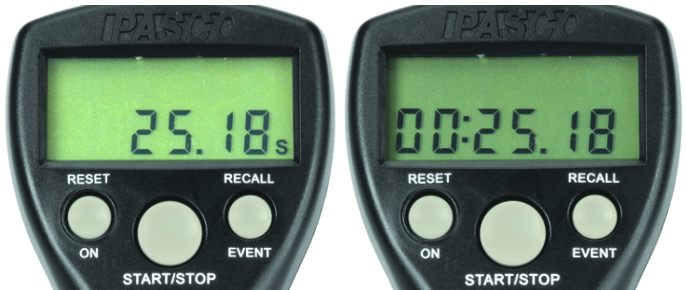
Figure 1. Decimal Seconds (left; default) and MG:SS:SS (right) display modes.
