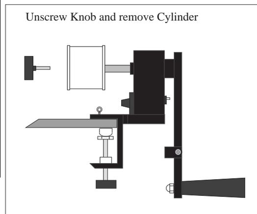
**Figure 7 Clamp to Table and Remove Cylinder**
