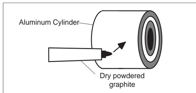
**Figure 4 Lubricate Cylinder**
