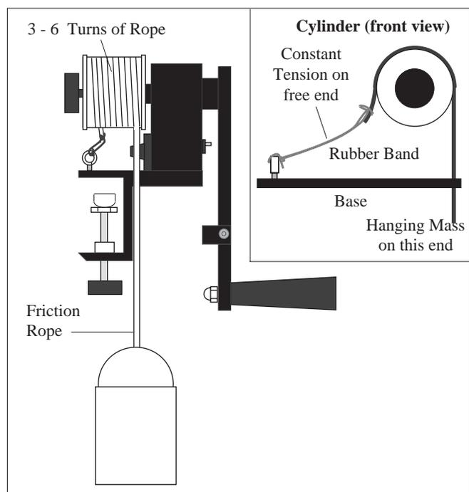
Figure 9 Add Friction Rope and Hanging Mass
