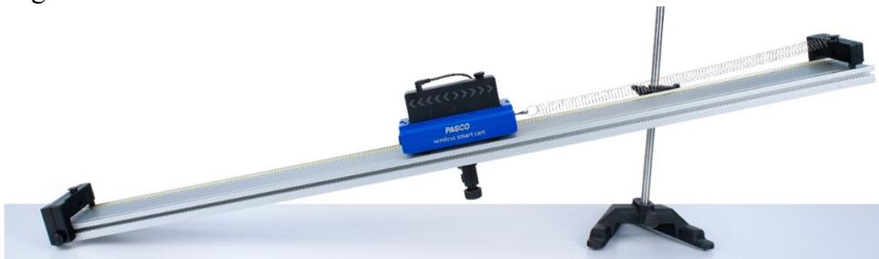
3. Attach the hook to the Smart Cart force sensor. Attach the Smart Cart Vector Display to the Smart Cart on the side opposite the accessory port. Connect the Vector Display to the Smart Cart accessory port using the connecting cable.
