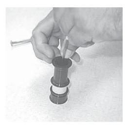
7. Hold the sight in the center of the piston with the screwdriver tip and firmly push it into the groove until it snaps into position.
