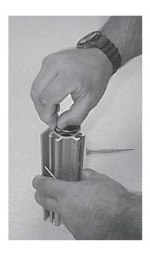
4. Pull the large black washer out of its groove to enable access to the piston.
