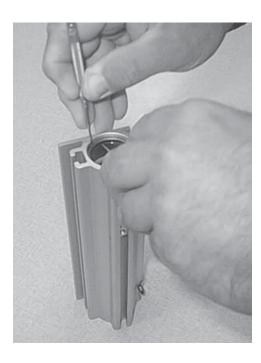
2. Pry the tab away from its seated groove of the cylinder and pull upward.
