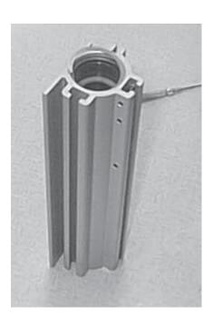
3. Slowly rotate the ring out of its groove until it is removed from the cylinder.
