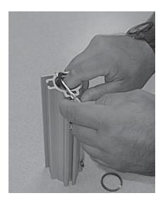
5. Pull up on the trigger and remove the piston.
