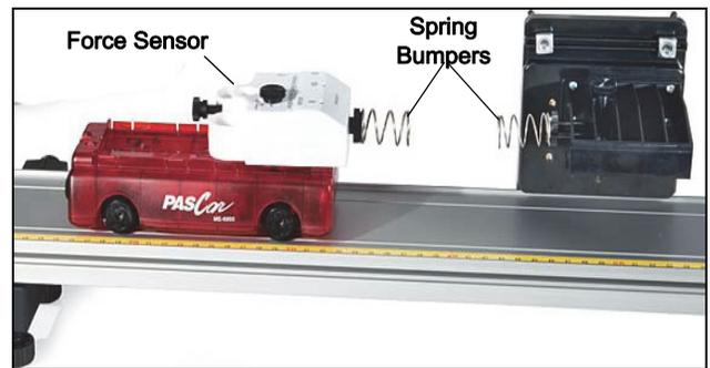
If the Bracket is mounted so that the flat surface of the Bracket Platform faces upward, a Force Sensor mounted on the Bracket Platform will be level with a Force Sensor mounted on a PASCO cart.
