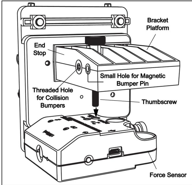
Screw the thumbscrew into the force sensor until the sensor fits snugly against the bottom of the Bracket platform.
