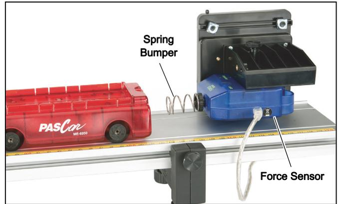
Also, a bumper mounted on the front of the Bracket Platform would be level with a Force Sensor mounted on a PASCO cart.
