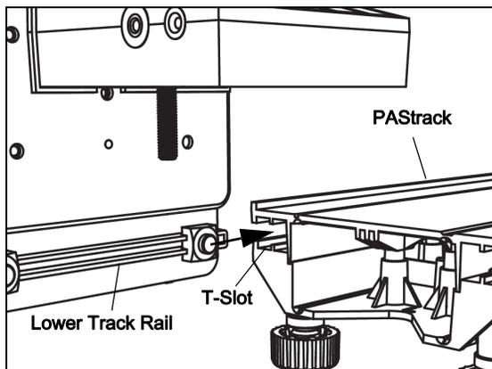
The Bracket can be fastened to the T-slot on either side of a PASCO track. The top edge or the bottom edge of the Bracket can be attached to the track. If the Bracket Platform faces down, then a Force Sensor mounted under the platform will be level with a PASCO cart on the track.
