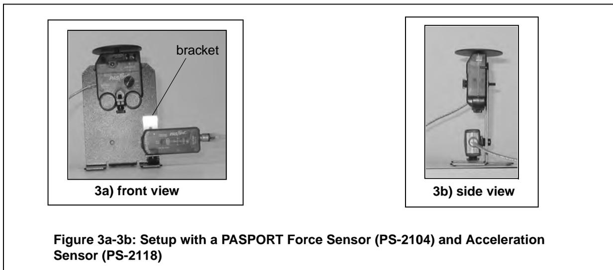
Hold the bracket against the side hole in the Force Sensor Stand. Insert a screw into the back of the Acceleration Sensor and mount to the back of the stand. Insert another screw into the bottom of the Acceleration Sensor to hold the sensor in place.
