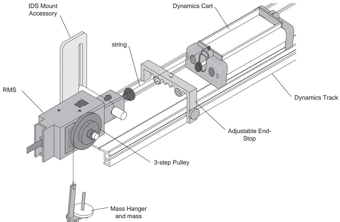
**Equipment Setup Using RMS Like a Smart Pulley**
