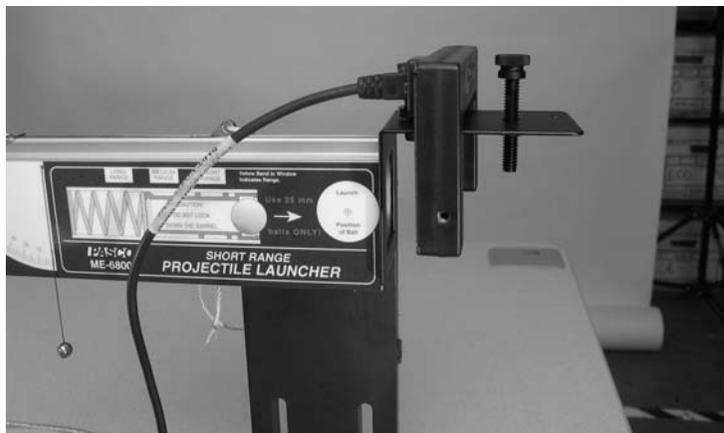
5. Connect a photogate as shown to measure the initial speed of the fired ball (optional). Since the photogate beam passes through the center of the ball's path, the velocity of the ball is calculated by the following equation:
