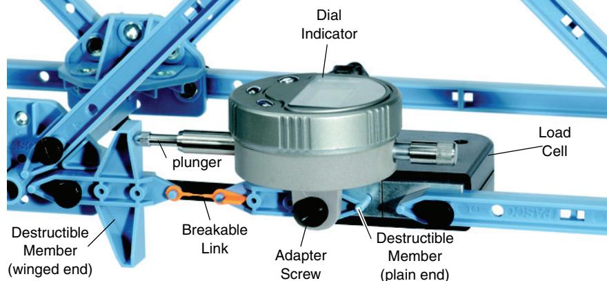
As each slotted mass is added, the stretch of the Breakable Link is measured by the Dial Indicator of the Displacement Sensor. The tension (**stress\***) is measured by the Load Cell. The displacement (**strain\*\***) suddenly increases when the Breakable Link is stretched beyond its elastic limit. The metal plate keeps the bridge structure from collapsing catastrophically if the Link does fail..
