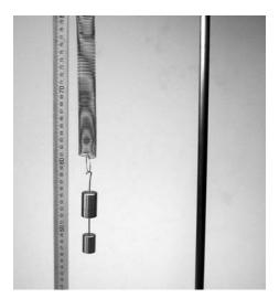
2. Place a hooked mass or mass hanger on the bottom on the spring.
