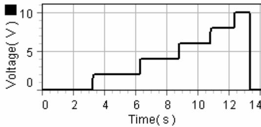
The standard step function requires each step to have the same width. This custom program allows each step to have a different width.
