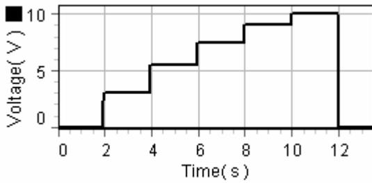
The standard step function requires each step to have the same height. This custom program allows a different height for each step.
