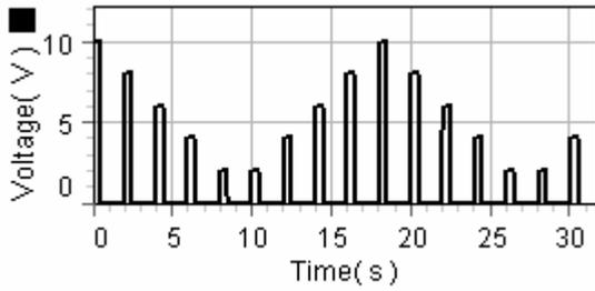
This program simulates Pulse Amplitude Modulation (PAM), which is used to introduce the modulation scheme known as Pulse Code Modulation.
