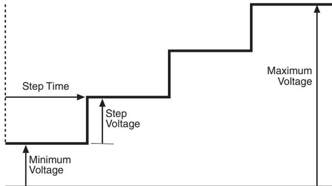
The *signs* of the Step Time and Auto-repeat parameters (+ or -) determine the shape of the wave. Step Time is positive for an ascending stair or negative for a descending stair. Auto-repeat is positive for a stair that goes in one direction (either up or down) before repeating or negative for stairs that alternate directions.
