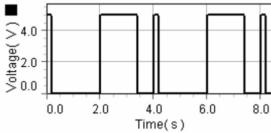
The standard square-wave function allows you to change the duty cycle, but all the pulses must have the same width. With this custom program you can create almost any pattern of pluses (including Morse code).
