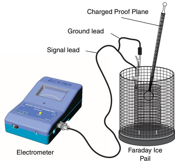
By touching the proof plane to a surface, it will acquire the same charge distribution as the surface. By measuring the charge on the proof plane, the charge density on the surface can be determined. The greater the charge on the proof plane, the greater the charge density on the surface where the proof plane made contact.
