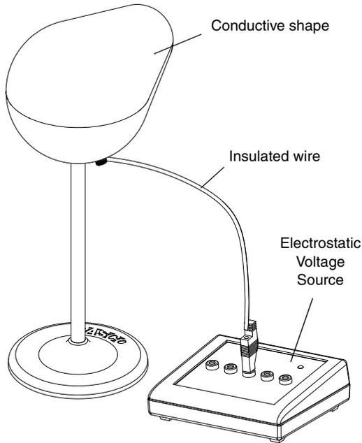
If you are using the PASCO ES-9078 Basic Electrometer to measure voltage, connect the electrometer ground terminal (GROUND) to the black ground terminal on the voltage source.
