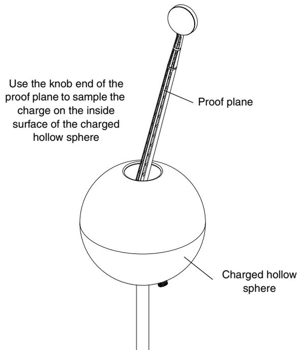
Remember to lower the charged knob end of the proof plane into the Faraday Ice Pail in order to measure the charge density inside the hollow sphere.
