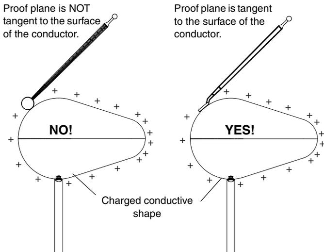
Is the charge density at the larger rounded end greater than, the same as, or less than the charge density in the tapered area? Is the charge density in the tapered area greater than, the same as, or
