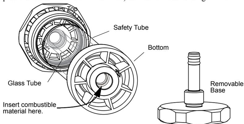
3. Use the loading/cleaning rod to push the material up into the lower part of the glass tube. Carefully remove the loading/cleaning rod without pulling the material out of the lower part of the glass tube.
