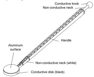
**NOTE:** Oil build-up on the non-conductive neck can affect results. Clean with alcohol before using.
