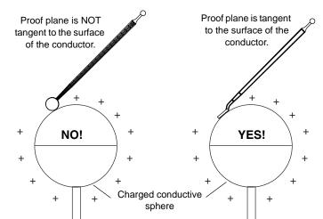
**NOTE**: To accurately sample charge density, the conductor should be considerably larger than the disk of the proof plane and have a relatively large radius of curvature at the point from which the sample is taken. However, the proof plane can be used to test for charge polarity on conductors of any shape.
