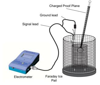
By touching the proof plane to a surface, it will acquire the same charge distribution as the surface. By measuring the charge on the proof plane, the charge density on the surface can be determined. The greater the charge on the proof plane, the greater the charge density on the surface where the proof plane made contact.
