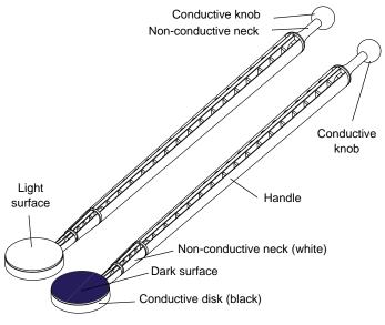
Briskly rub the light and dark surfaces of the two charge producers together. The disk with the light surface will acquire a positive charge; the disk with the dark surface will acquire a negative charge. Rub the light surface charge producer against the proof plane. The white disk will acquire a negative charge, while the disk of the proof plane will acquire a positive charge.
