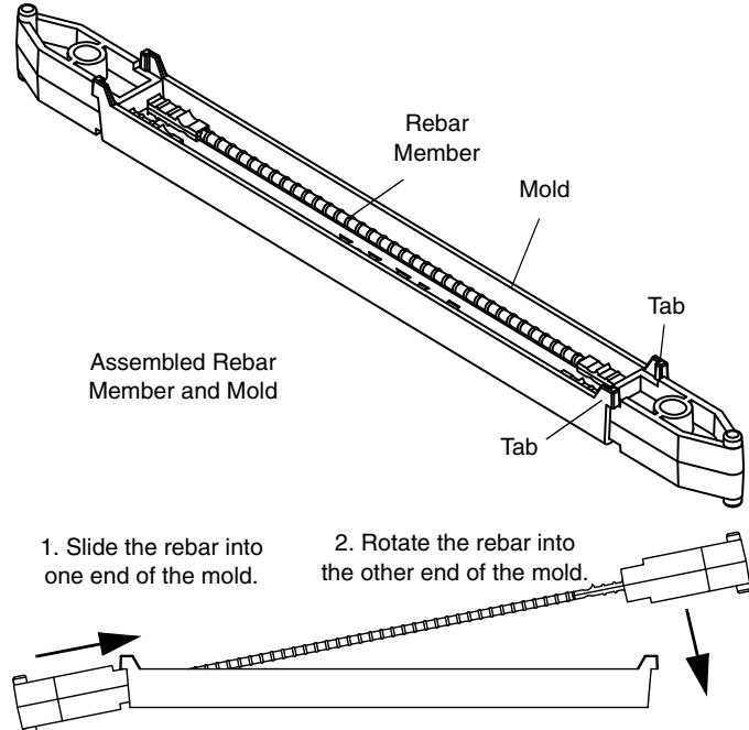
**Caution:** Do not stretch the rebar member with more than 100 N of force (the hanging weight of about 10 kg of mass).
