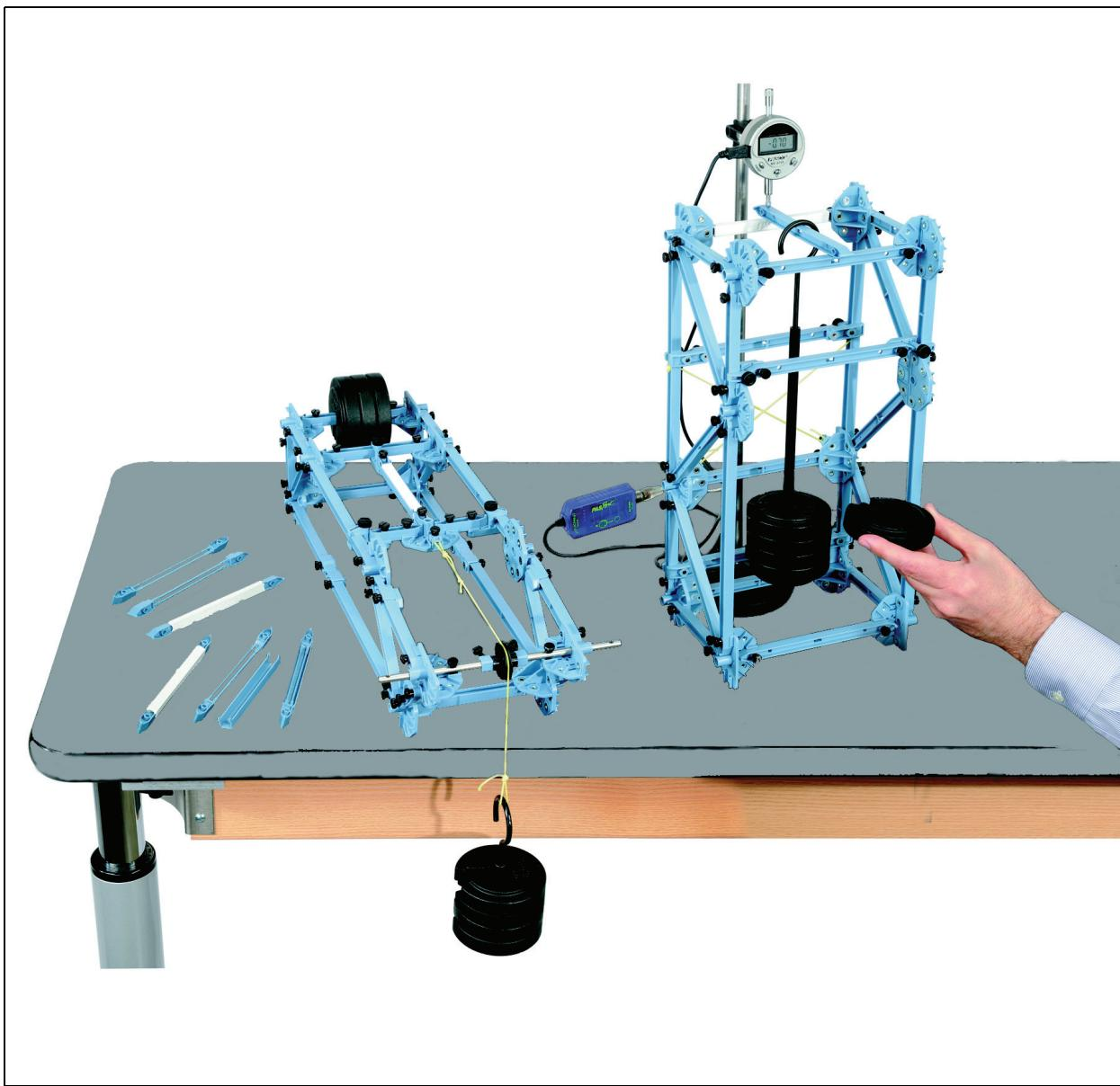
The cover page shows the ME-7009 Cast Beam Structures Set models of a Tension Fixture (left) and a Test Fixture (right). The tension fixture uses a hanging mass to pre-stress a cast beam member, and the test fixture can be used after the cast beam member has dried and the mold has been removed. A hanging mass applies a load to the cast beam, and a displacement sensor measures the amount of deflection.
