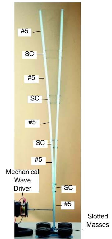
Place slotted masses (such as those from the ME-7566 Large Slotted Mass Ses) on top of the Flat Connectors to stabilize the resonance beam.
