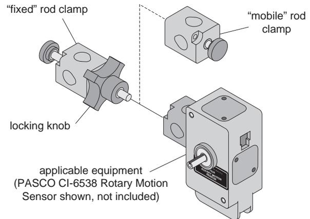
**Figure 3: Alternate Use for the Adjustable Angle Rod Clamp**
