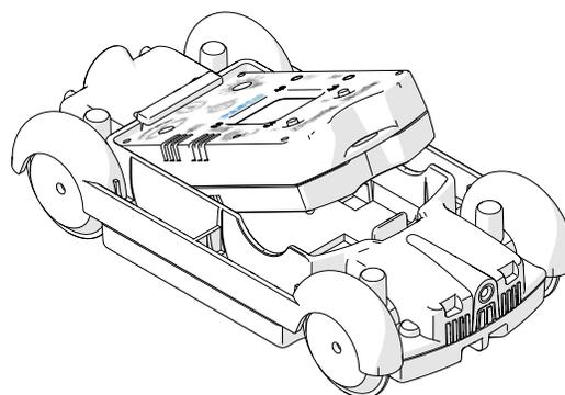
1. Insert the top side of the //code.Node into the cart bay face up.
