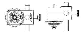
The Pivot has two support rod holes that fit rods up to 0.5 inches (12.7 mm) in diameter. It is possible to mount the Pivot horizontally on a support rod with the Threestep Pulley facing up or facing sideways. You can mount the Pivot vertically with the pulley facing forward.
