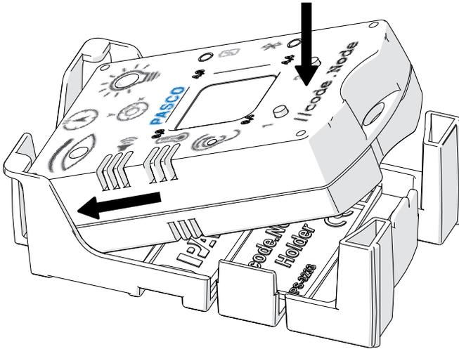
1. Insert the top side of the //code.Node into the Holder face up.
