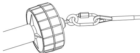
Figure 2. Carabiner attached to the transparent cover eye bolt on the Wireless Optical Dissolved Oxygen sensor.
