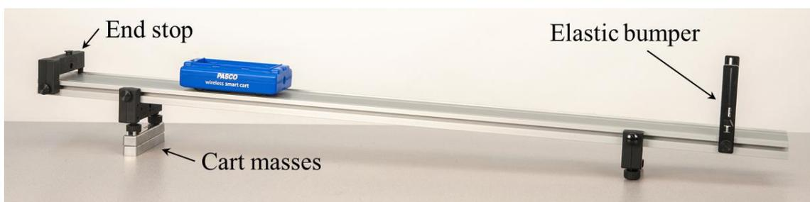
Figure 1: Smart Cart on Inclined Track
