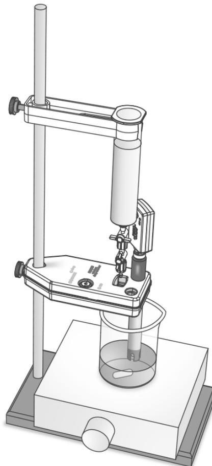
*NOTE: The top valve controls the flow rate and the bottom valve turns the flow on and off.*
