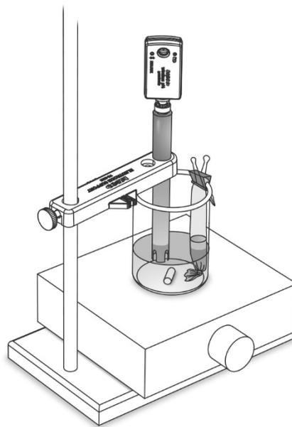
Figure 2: Secure the bag to the beaker with the binder clip
