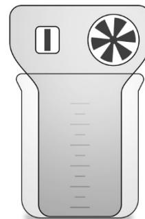
Figure 1: Set sensor in beaker
