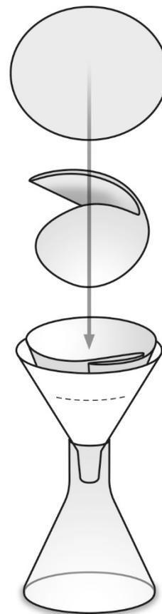
Figure 1: Flask filter
