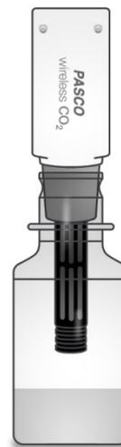
Figure 1: Seal the bottle with the sensor
