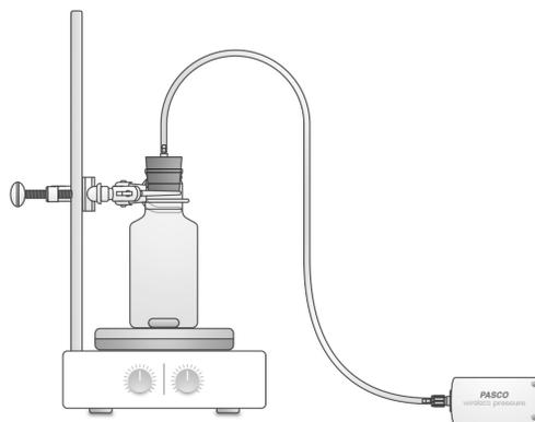
Figure 1: Setup with stirrer
