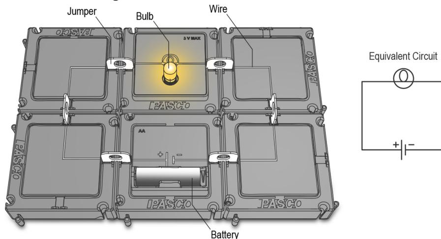
1. Connect a battery, bulb, and four wire corners together to create the circuit in the diagram.
