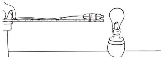
7.  Make sure the meter stick is aligned with the center of the bulb. The distance separating the meter stick and the bulb should be around 10-20 centimeters depending on the wattage of the bulb.
