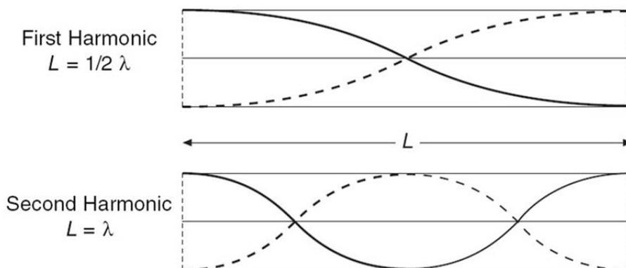
Figure 3: Modes of Vibration in an Open Tube of Fixed Length
