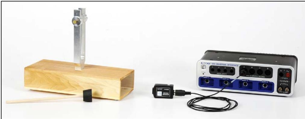
Figure 3: Tuning Fork and Sound Sensor
