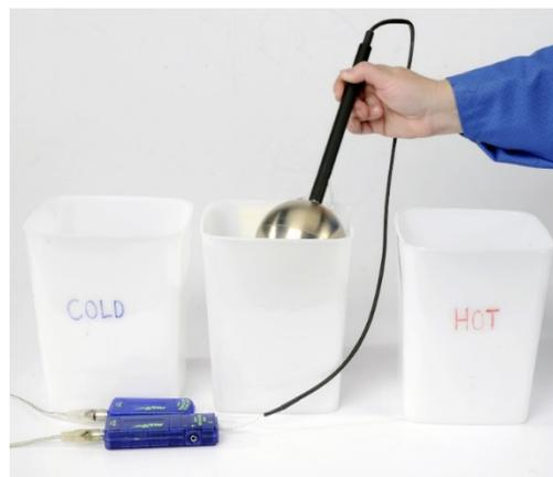
Figure 3: Three Different Temperature Baths
