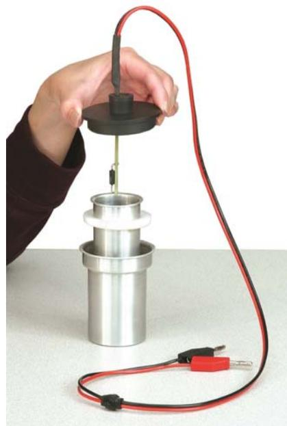
Figure 2: Calorimeter Assembly
