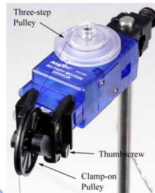
Figure 3: Adjusting Angle of Clamp-on Pulley
