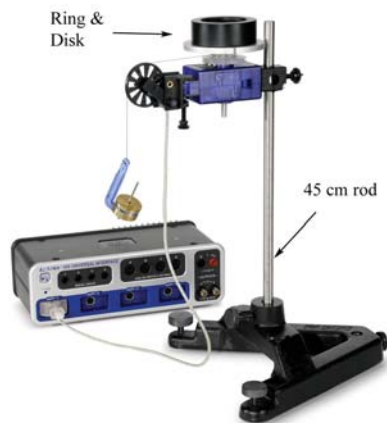
Figure 1: Measuring the Rotational Inertia of Ring and Disk
