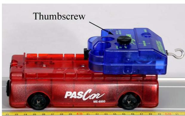
Figure 3: Attaching Sensor to cart
