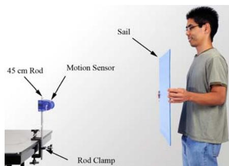
*Figure 1: The large blue "sail" from the ME-9595 Car Sail is used as a target to improve the graph results using the Motion Sensor.*
