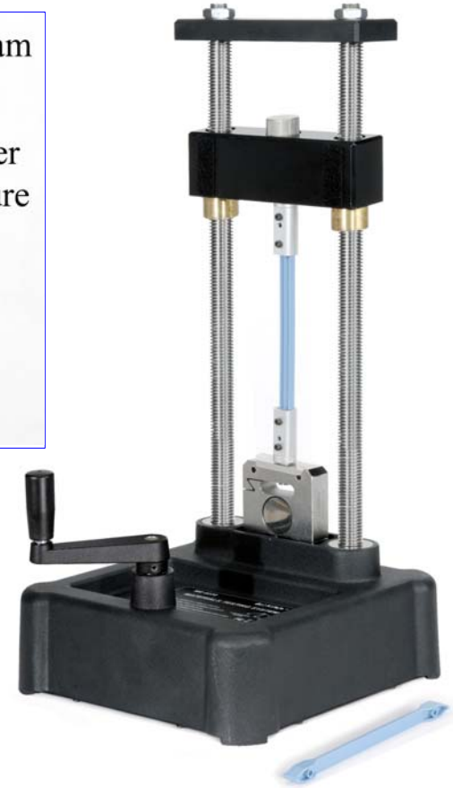
Figure 1. Tensile testing plastic beams.
