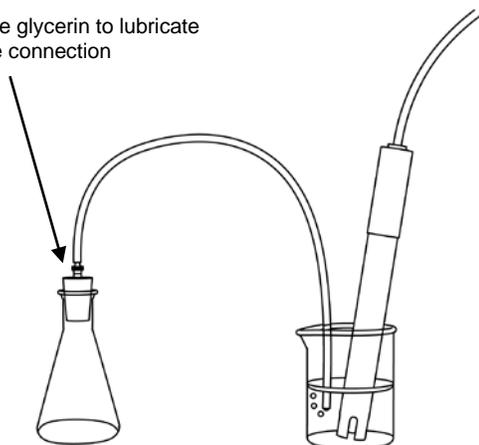
13.  Pipet 4 mL of 1.0 M hydrochloric acid ( $\text{HCl}$ ) into the Erlenmeyer flask, and immediately stopper the flask.
