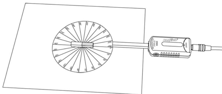
28.  Position the magnetic field sensor's tip at the 0 degree line on the template as shown in the diagram. The closer you place it, the stronger the field will be; keep the sensor the same distance from the magnet and in line with the circle.
